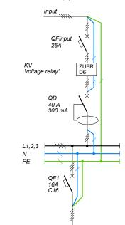
correct operation of ZUBR D6. it is enough to connect eutral conductor to one of the zero terminals (4 or 8).
