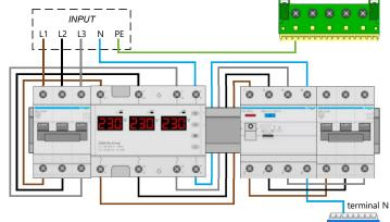
Scheme 3. Wiring diagram
