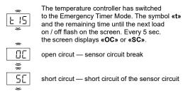
Possible cause: damage to the sensor and its circuit.
