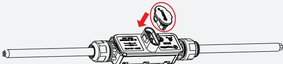
*Note: Under the circumstance that need to remove the inverter AC cable from 3P-AC bus connector, please use the 3P-AC connector unlock tool and insert the tool into the side of AC port to remove.*
