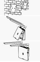
Option 2: Place the DTU on table. Please make sure the antennas are vertical to the table.
